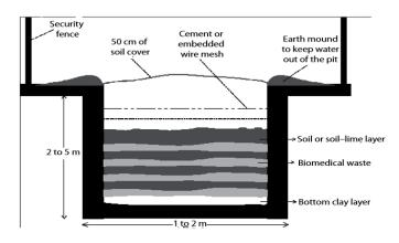
Fig. 2. Construction of a pit for onsite waste burial (7)
